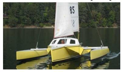
coast where he now resides. It is based on the use of more recent designs of catamaran hulls that are larger in volume than say the Hobie 16. His study plans are in fact drawn around the Quattro 16 that is molded with a long built-in fin keel and no dagger boards, which is a smart move for trimaran
