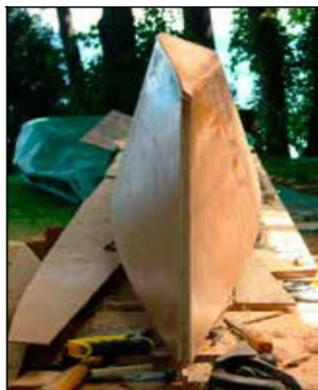
Waters built MAGIC under a temporary rain shelter sized to just fit the project. The cockpit, mounted here on the main hull, is rectangular, making it simple to build while maximizing useful space.
