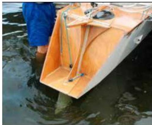
**Far Left:** The entire rudder assembly is attached via a deck-mounted hinge, allowing the rudder to be raised easily. **Left:** When lowered the unit's lower flange mates into the bottom planking, allowing the spade rudder to operate efficiently and in very little turbulence.
