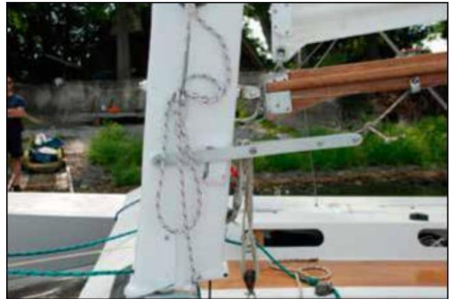
**Left:** The daggerboard trunk's top is flush with the sole, making the cockpit self draining. The board is shown here partly retracted and pivoted forward for working in the shallows: bungee cords hold it in place.
