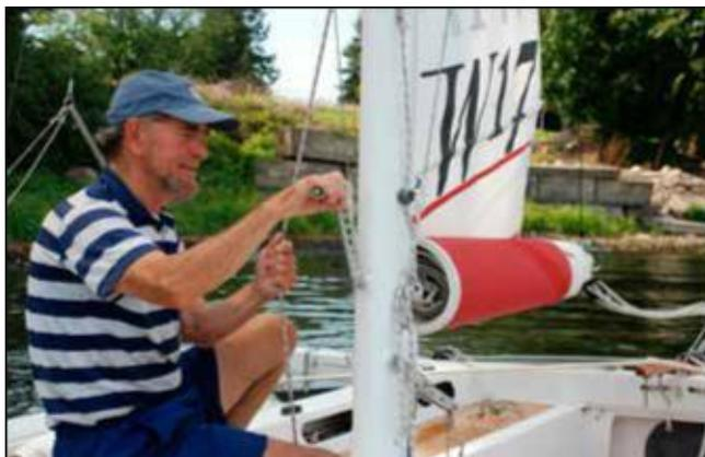
**Designer and builder Mike Waters demonstrates the ease with which the mainsail furls around the boom. The handle stows in a handy tool locker built into the forward aka fairing at the heel of the mast.**
