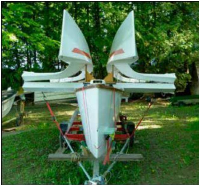
**Hinged akas allow the amas to fold up for transportation or storage. When folded, the amas rest on a purpose-built brace set on the beam top, relieving strain on the hinges. The flat-bottomed hull transports easily on a flatbed trailer.**
